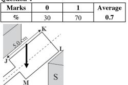
Using the 'right hand slap' rule, the force was vertically down as shown. It should be noted that the vector arrow originates from the point of action of the force.
